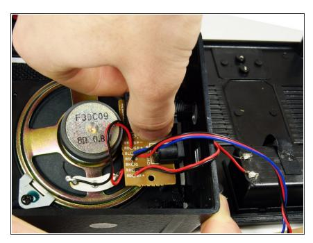
Grab the headphone jack from inside the case and pull it toward the speaker until you can fully remove it from the device.
