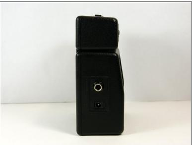
Use a 9/16" socket to remove the nut around the headphone jack. Be careful to not lose the washer.
