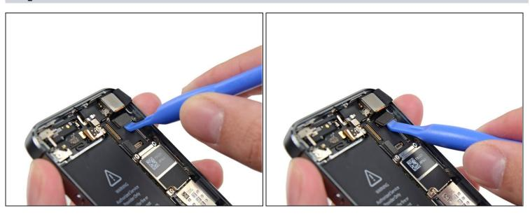
• Using a plastic opening tool, disconnect the rear-facing camera cable connector from the logic board.
