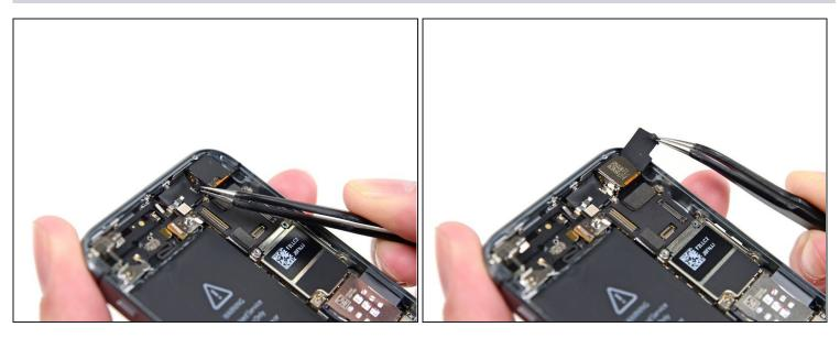
• Using a pair of tweezers, flip the rubber camera cover out of its clip, and toward the outside of the rear case.
