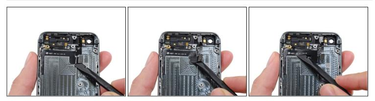
• Slide the flat end of a spudger under the upper component assembly cable to free it from the rear case.
