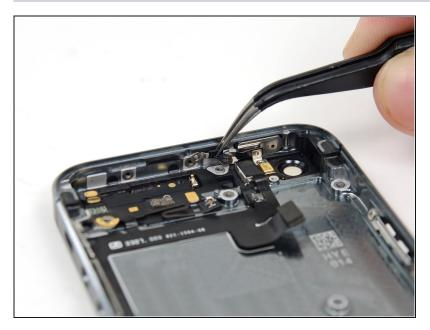
• Remove the logic board antenna bracket.
