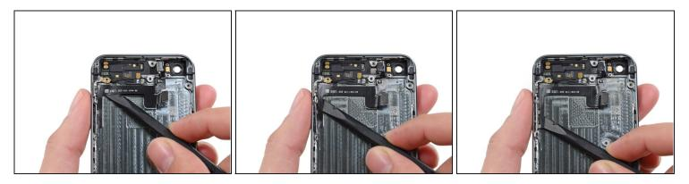
• Run the flat end of the spudger under the portion of the cable near the volume control buttons.
