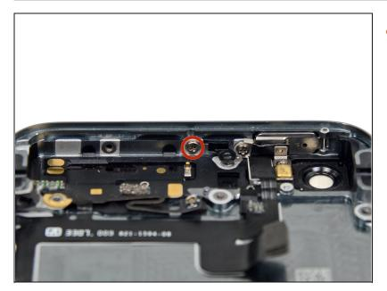
Remove the 1.3 mm Phillips #000 screw securing the logic board antenna bracket to the rear case.
