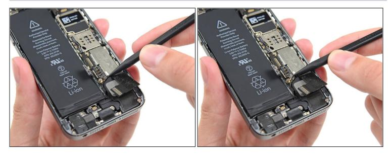
• Use the tip of a spudger to pry the antenna cable up from its socket on the logic board.
