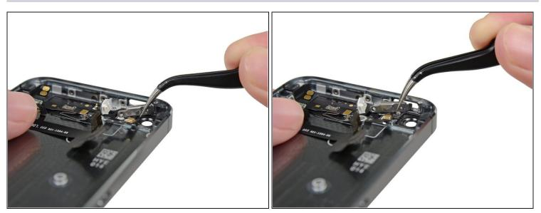
• Unclip the power/sleep button bracket hinge from the post holding it in the iPhone.
