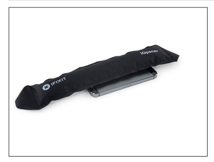
If any of the adhesive strips broke off and the battery remains stuck to the rear case, <u>prepare an iOpener</u> or use a hair dryer to heat the rear case directly behind the battery.
