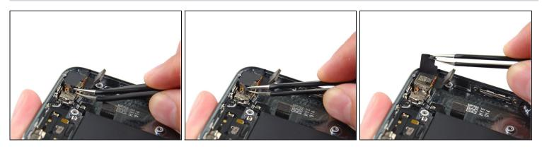
• Using a pair of tweezers, flip the rubber camera cover out of its clip and toward the outside of the rear case.
