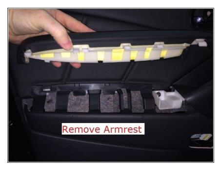
Pry up the arm rest to expose the second hidden screw (total of 3).
