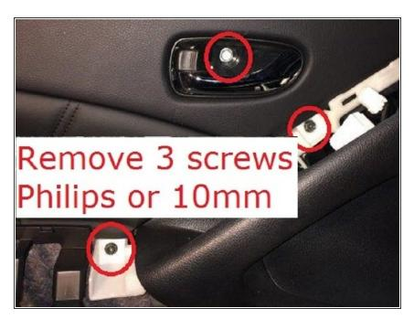
Now you can remove all three hidden screws with the 10mm socket or philips screw driver.
