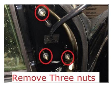
Remove the three nuts holding the mirror on to the door. Depending on the age of your vehicle, you may want to clean off the remaining area so the new mirror seals good.
