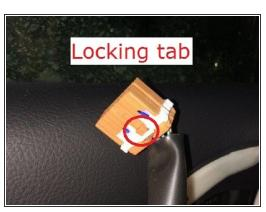
Pry out the door lock and window control panel. Disconnect all connectors on the back side.
