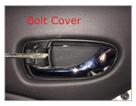
Expose one of three screws by prying the door handle trim plate out.
