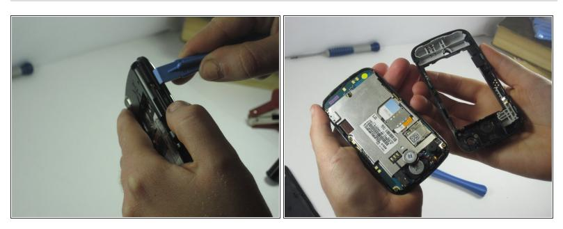
Using a prying tool, separate the frame of the phone.
