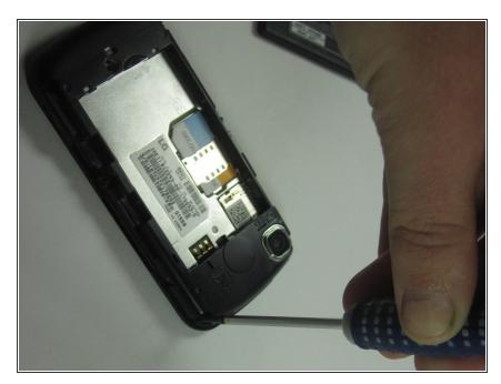
Use a Phillips #0 screwdriver to remove the six screws around the edge of the device.
