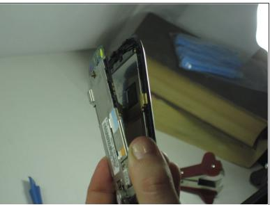
Using a prying tool, separate the screen from the motherboard.
