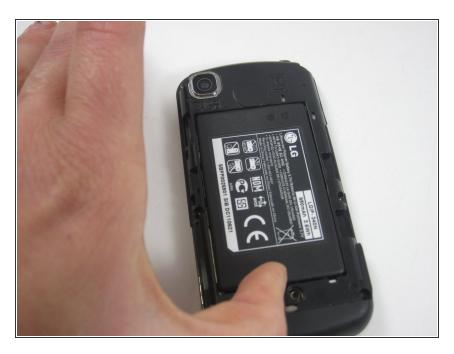
Remove the battery by gently lifting it up from the bottom.
