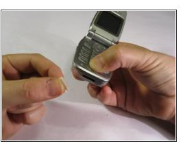
• The phone may have a rubber insert in the bottom of the phone (see picture). If this rubber insert exists, remove it from the bottom of phone and set aside.
