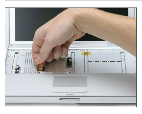
Use the orange plastic loop to disconnect the trackpad cable.
