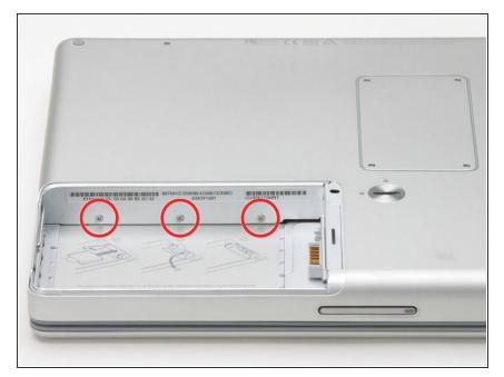
Remove the three small Phillips screws from within the battery compartment.
