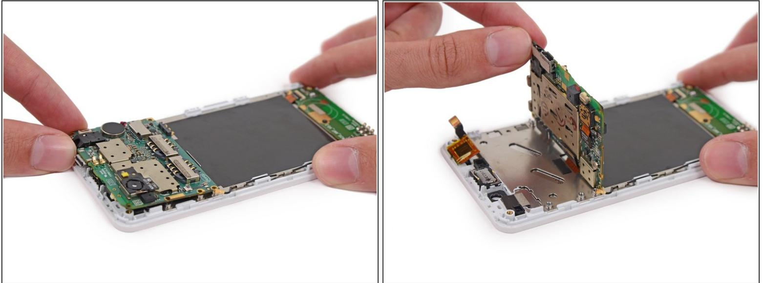
**⚠** Do **not** try to remove the motherboard just yet, as it is still connected to the display assembly by the display data cable.
