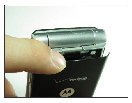
Using your finger, press down on the clip holding the back cover on.
