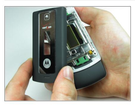
If the casing has not popped off of the body, remove it carefully from the the phone.
