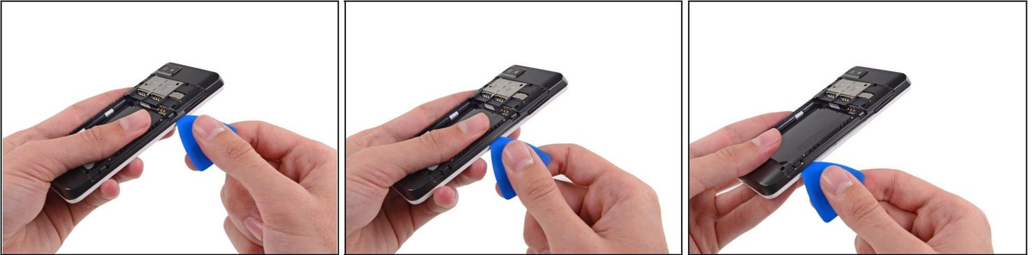
ⓘ The midframe is secured to the display assembly by several small plastic clips.
