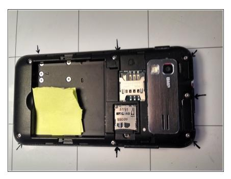
Using the Phillips #00 screwdriver remove the seven screws indicated here.
