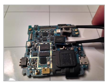
The camera can be easily removed from the motherboard by pulling up on the board pop connector.
