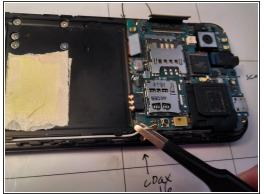
• In order to remove the motherboard remove a single screw with the phillips #00 screwdriver, gently pry up the two pop connectors on the board, and finally pull off the coaxial cable.
