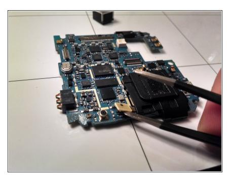
The speaker is also easily removed by pulling up on the pop connector.
