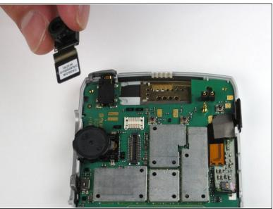
Take out the camera and attached chip with the iPod removal tool. Carefully pry the chip off its connection and the camera will come out too.
