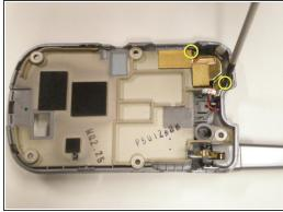
Remove both screws with a #00 philips screwdriver.
