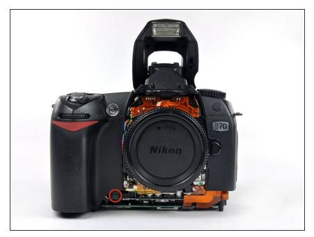
Remove the 4.2 mm Phillips screw securing the lower edge of the grip to the front of the D70.
