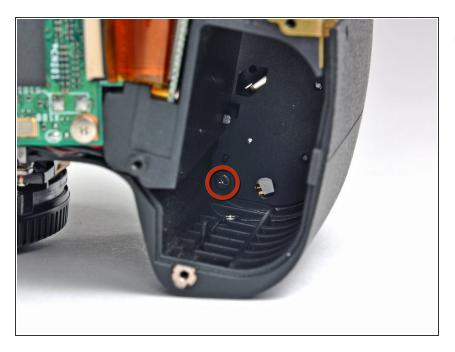
Remove the 5.7 mm Phillips screw in the top corner of the battery compartment.
