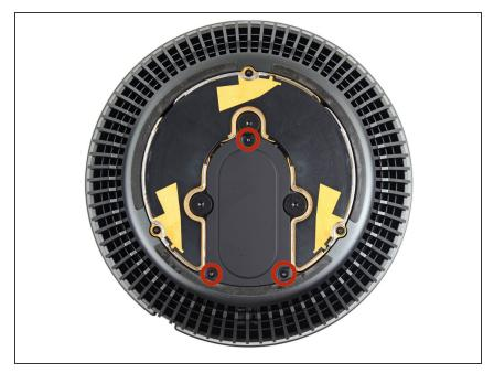
Remove the three 3.7 mm T4 screws securing the metal cover to the AirPort board bay.
