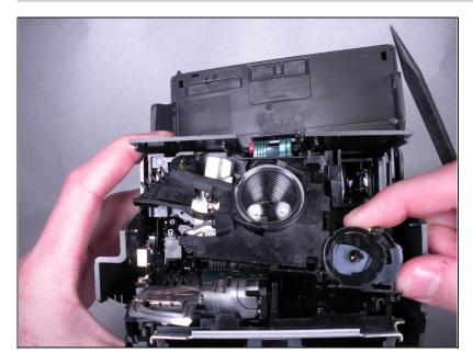
Remove the lens plate by pulling down, then away from the camera.
