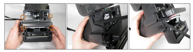
• Insert spudger in between face of camera and sides where the four tabs are located.
