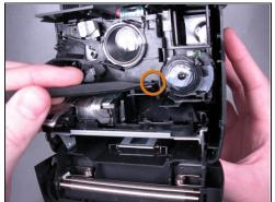
Release the two tabs that hold lens plate in position.
