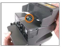
• Separate the flash section of the camera from the main body by unhooking the sides.
