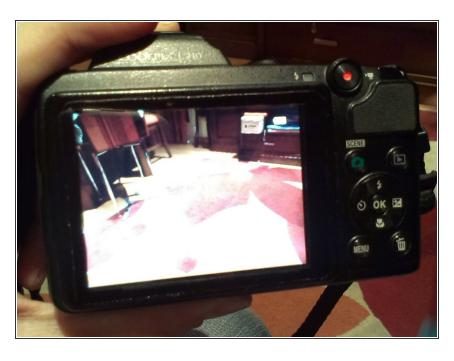
Re-assembly all the parts, and put back the screws. The reparation is DONE! Here you can see the display fixed and the outer window replaced by methacrylate part made by myself (I have one Dremel...) To reassemble your device, follow these instructions in reverse order.
