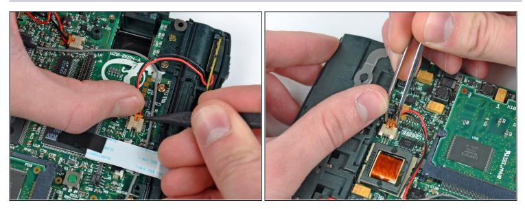
Before removing the stylus holder, disconnect the power button and backlight connectors from the logic board.
