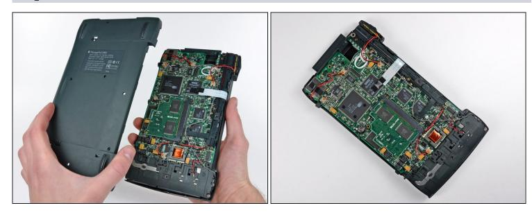
• After much (careful) wiggling and prying, the rear case lifts right off the Newton.
