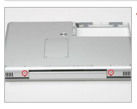
Remove the two Phillips screws from either side of the display hinge.
