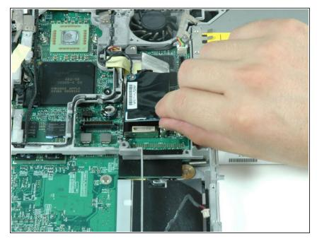
Disconnect the modem from the logic board by lifting the bottom edge of the modem. Don't remove the modem entirely just yet as it is still connected to the RJ-11 board.
