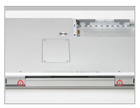
Turn the computer 90 degrees clockwise again, and remove only the bottom screw on either side of the hinge.
