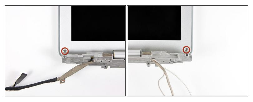
Remove the two T6 Torx screws in the lower left and lower right corners of the display securing the rear bezel to the display assembly.
