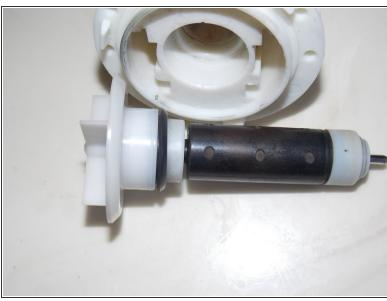
• For this discussion the core comprises of the following as one unit: rotary blade, lid, rubber seal, spindle and magnet. To remove the core, gently pry with a flat head screw driver all around the top edge and gently lift the core out of the case housing.
