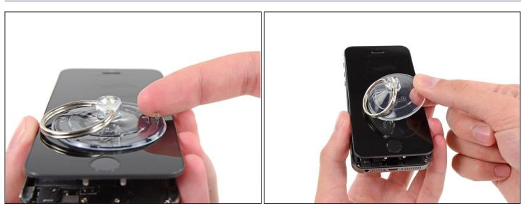
$\triangle$  Do not try to completely remove the front panel assembly from the rear case, as there are several delicate ribbon cables connecting them.
