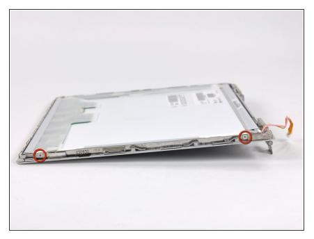
Remove the two 3.0 mm Phillips screws securing the LCD to the right side of the front display bezel.
