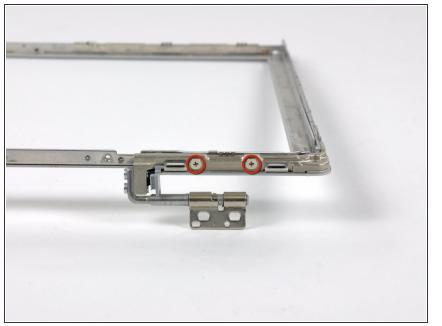
Remove the two 5.5 mm Phillips screws securing the left clutch hinge to the front display bezel.
