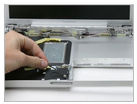
• Deroute the Airport Extreme antenna from the card slot and lower case, removing tape as necessary.
