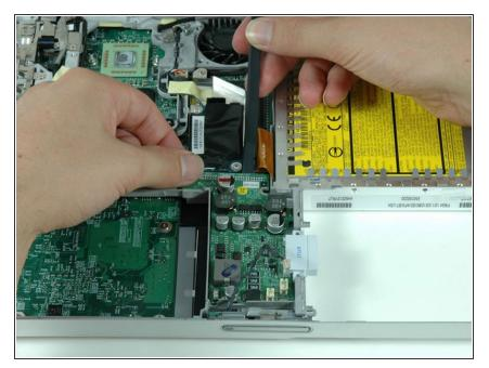
Use a spudger to pry up the end of the DC-to-DC board closest to the display and remove the board from the computer.
