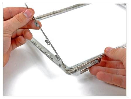
• Lift the bar section of the clutch hinge a bit and remove the entire clutch hinge from the front display bezel.
