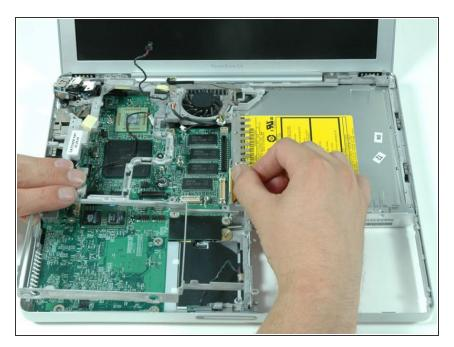
Pull back on the orange optical drive cable with one hand, and use your other hand to lift the front section of the metal framework over the optical drive cable.
