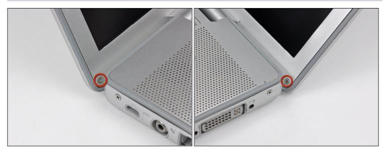
• Remove the two 6.3 mm Phillips screws near the lower left and right corners of the display.
