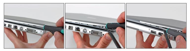
• Insert the flat end of a spudger between the rear display bezel and the plastic rim attached to the front display bezel near the lower right corner of the display.
