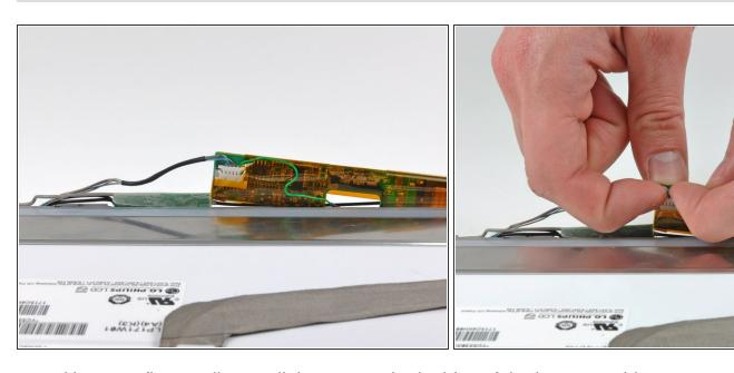
Use your fingernails to pull the ears on both sides of the inverter cable connector away from its socket on the inverter board.
