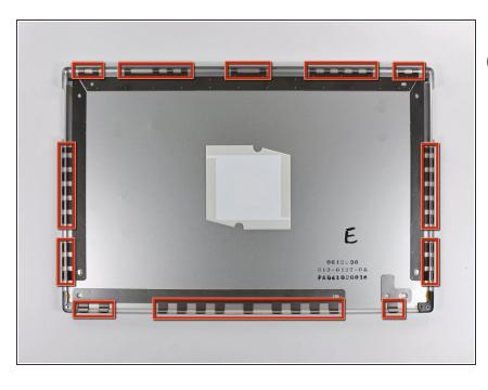
The picture at left (rear panel already removed) shows the locations of the metal clips (shown in red) that snap on to the front display bezel. In the next few steps, you will use a small flathead screwdriver to release these clips from a ridge around the perimeter of the front display bezel.
