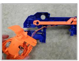
Remove the two 9.0 mm Phillips screws.
