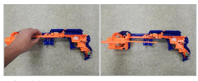
Remove the firing pin.
