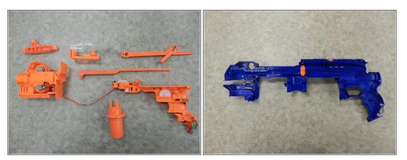
Once all the pieces are removed the right shell should be fully accessible.
