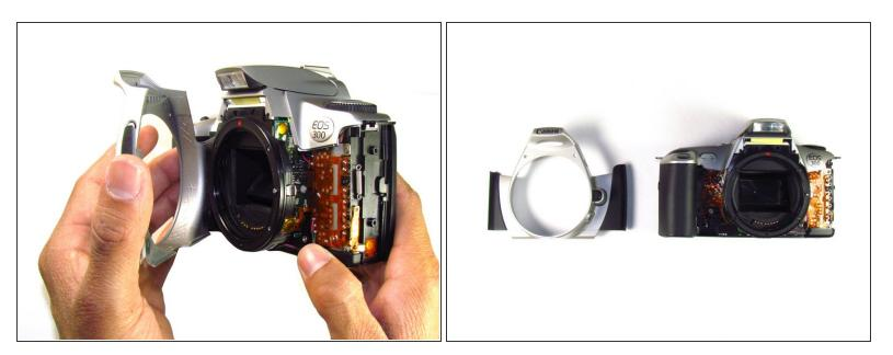
• Remove the front panel by pulling away from the side with the lever.
