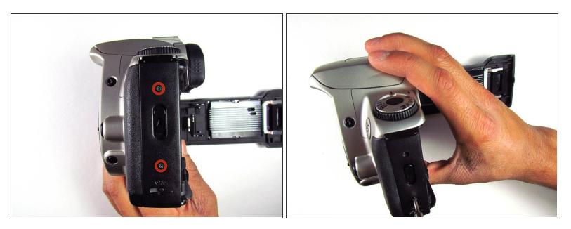
• Remove the two black 4.5mm screws above and below the latch.
