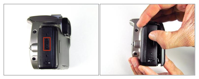
• Release the side latch to open the back panel.
