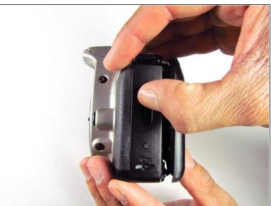
Release the side latch to open the back panel.
