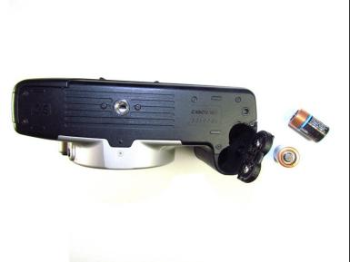
• Remove the batteries from the camera by sliding them out into your palm.
