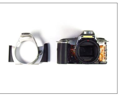
Remove the front panel by pulling away from the side with the lever.
