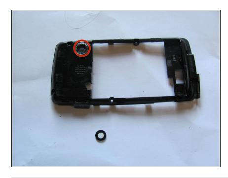
• Push the camera lens though its socket, from the inside out.
