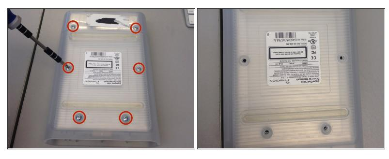
Remove the six silver screws using a small Phillips head screwdriver.
