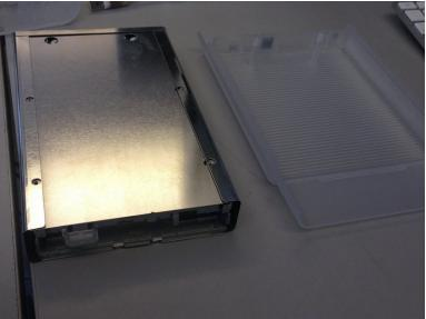
Slide the metal housing out of the plastic shell.
