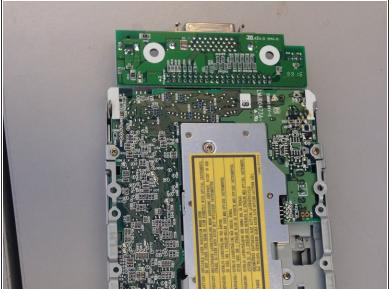
Slide disk drive out of metal casing.
