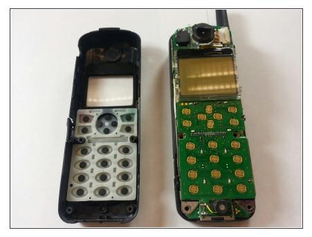
Separate the front plastic component from the motherboard component.
