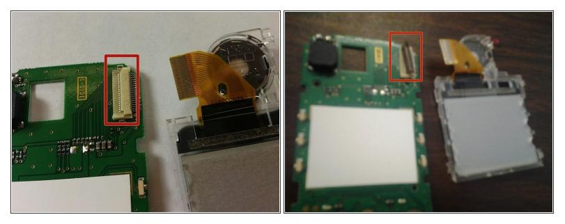
Remove the attached ribbon from the circuit board by prying open the gray plastic clip at the top right of the circuit board.
