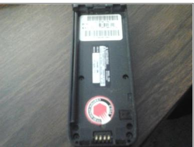
Begin disassembling the phone by removing the phone back cover and battery.
