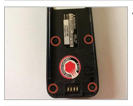
Firmly replace screws into the backing.
