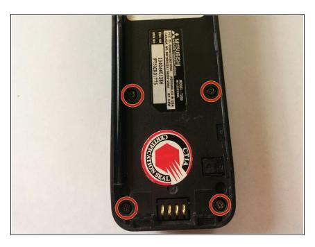
To remove the back plate, loosen and remove the four screws by using a #00 Philips head screwdriver.
