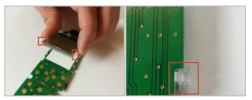
Unclip the four clips to remove the screen (connected to the clear plastic) from the circuit board.
