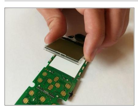
Clip the new screen onto the circuit board.
