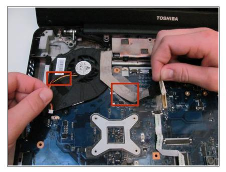
Remove the two cables from the fan.
