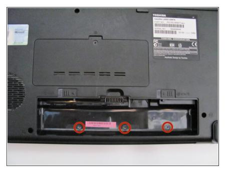
Remove the three 3mm screws from beneath the battery with a Phillips #1 screwdriver.
