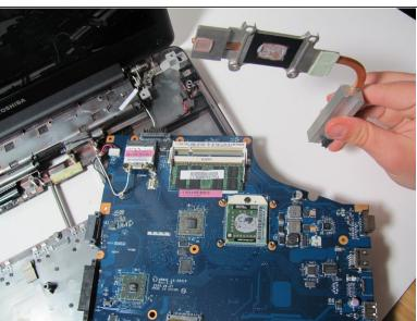
Remove the four Phillips #1 6mm single coil pickup screws from the cooling unit and remove the cooling unit.
