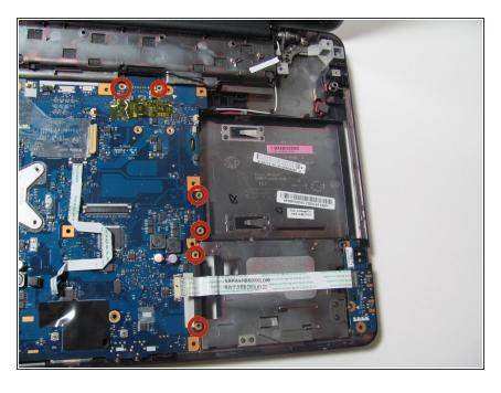
Remove the six 6mm screws from the motherboard with a #1 phillips screwdriver.
