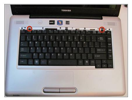
Remove the two Phillips #1 3mm screws underneath the plastic strip using a Phillips #1 screwdriver.
