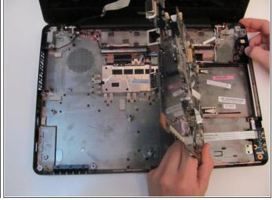
• Remove the motherboard with your hands by carefully lifting up and pulling out.
