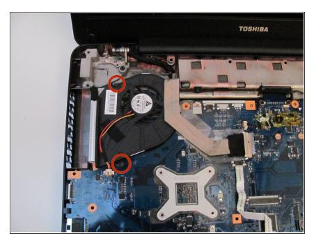
Remove the two Phillips #1 3mm screws from the fan using a Phillips #1 screwdriver.
