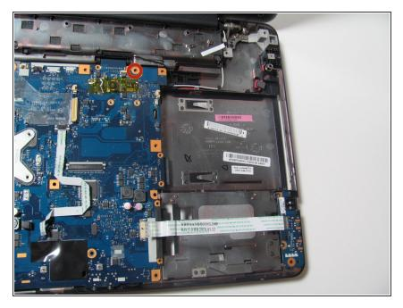
Remove the lone 10mm screw from the motherboard with a phillips #1 screwdriver.
