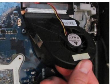
Lift up on the fan and remove it from the computer.
