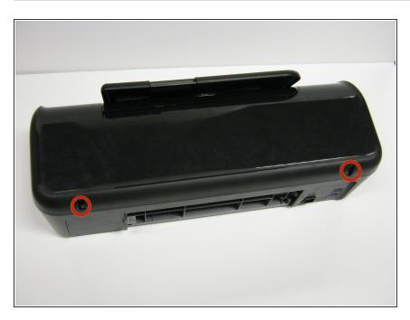
Remove the back two 14.0 mm Torx #10 screws.
