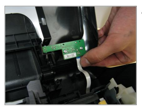
Remove the strip that connects the printer to the front cover.
