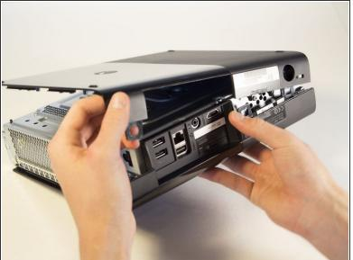
Push the spudger into the crevice. Slide the spudger along the vertical crevice to detach the last clip. The bottom body should slide off after this.
