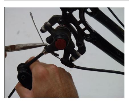
Tighten the screw on the desired location along the cable with the same 5mm allen wrench.
