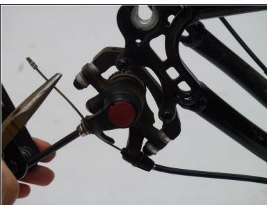
While holding onto the brake cable, unscrew the screw that holds the brake cable in place using a 5mm allen wrench.
