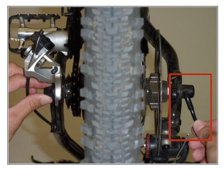
Begin loosening the tire by turning the quick release handle.
