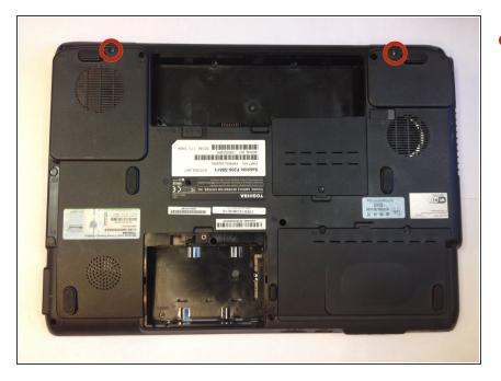
Remove the two 4mm Phillips #1 screws located between the screws removed in the last step.
