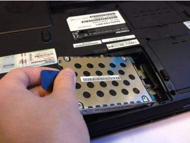
Grab the black tab attached to the hard drive and pull it to the left with a medium force until it pops out of its socket.
