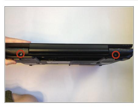
Remove the two 8mm Phillips #1 screws from the back side of the laptop.
