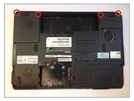
Remove the four 8mm Phillips #1 screws located on the corners below the monitor.
