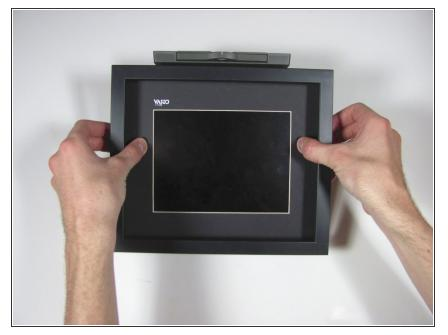
• Lift up the frame with your fingers and push down the rest of the device with your thumbs.
