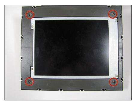
Remove the four 7mm Torx T6 screws.
