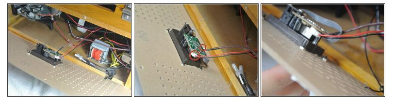
Gently remove the back of the device. It should be connected by two wires.
