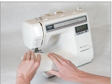
Pull off the storage area beneath the needle.
