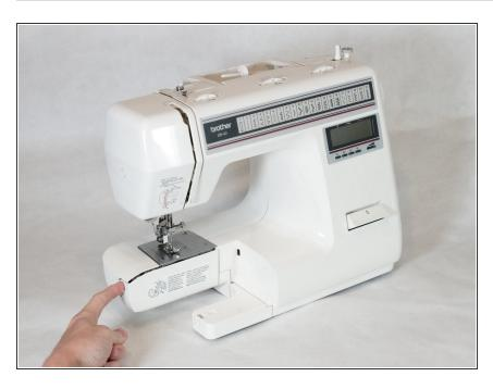
• Flip open the tab below the needle.
