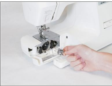
Pull on the end of the rectangular tab on the bobbin case. This will pop off the bobbin and bobbin case.
