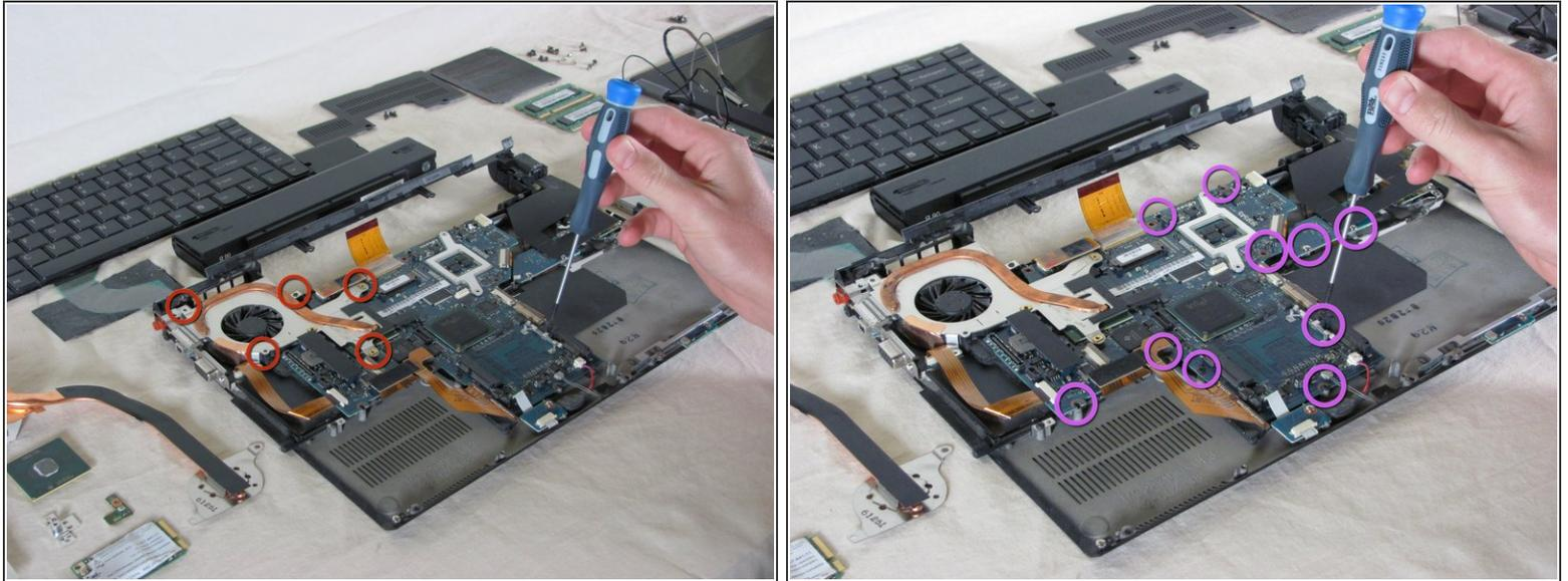
**⚠ Caution:** When removing the fan, be careful to not tear the attached ribbon cable.
