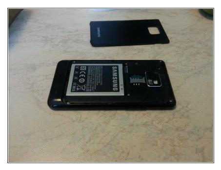
Remove battery door and battery
