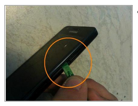
Use a plastic tool to separate the rear frame from the front
