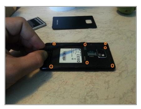
Remove all screws on the back of the plastic frame
