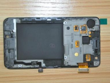
Remove the USB connector by unscrewing the two screws. Reinstall the new display starting from this step to number one on the procedure. To reassemble your device, follow these instructions in reverse order.
