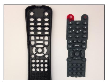
Remove plastic molding attached to the top half of the remote casing
