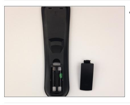
Remove the lid encasing the batteries
