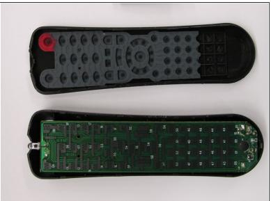
Using a flat head screwdriver pry open the remote
