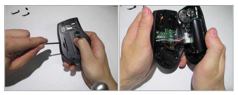
Pry the center of the mouse apart using a spudger to separate the upper and lower housing of the boards.
