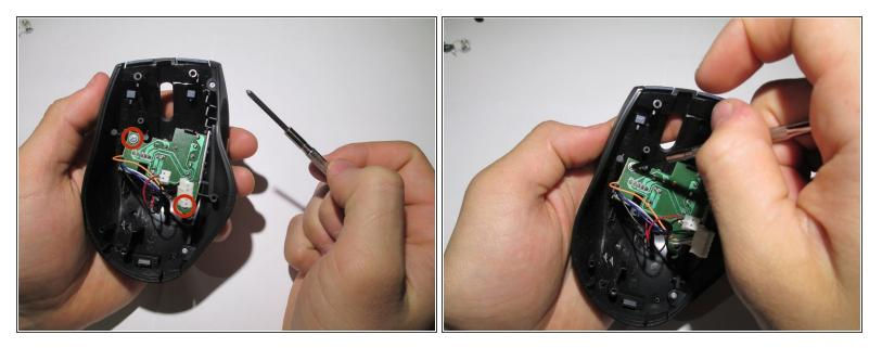
• Take the upper housing of the mouse and remove the two screws that hold the board in place.
