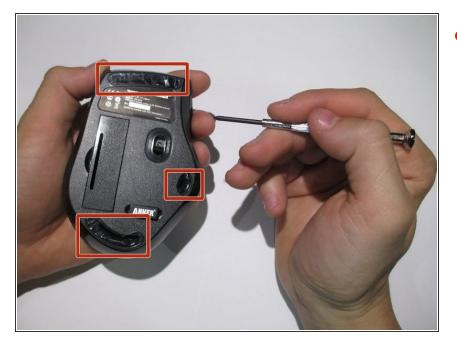
Use a spudger to gently pry off the stickers to reveal the location of the four screws.
