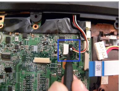
Disconnect the audio cable from the system board using the spudger tool.
