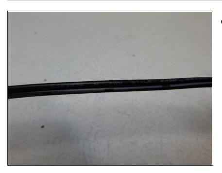
Take note of the wire labeling. Each wire has either a Stripe or Text. When lining up the wires after cutting, it is critical that you keep Stripe with Stripe, and Text with Text. Failure to do so will result in damage to the device.
