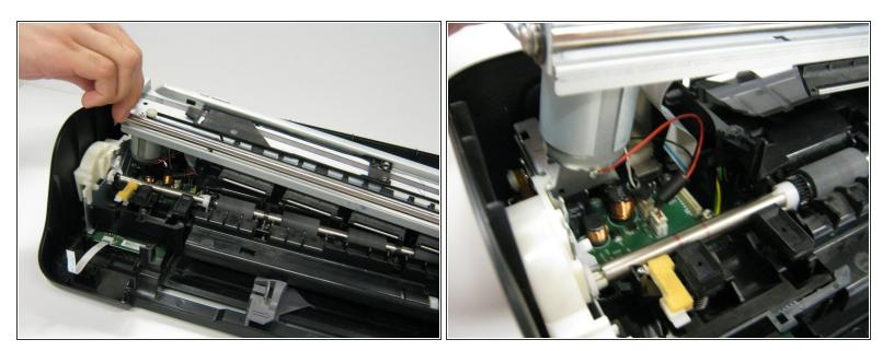
A Lift the rail carefully as a strip and motor will be connected to the bottom part of the printer.
