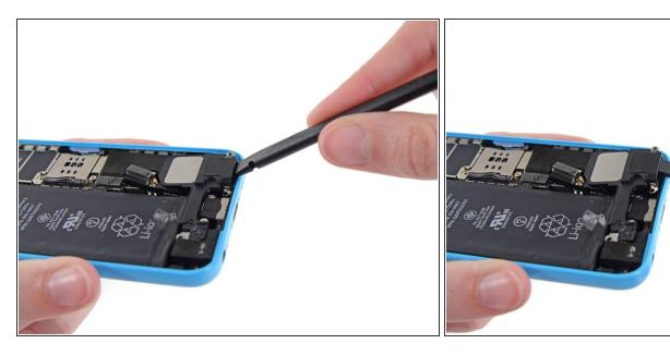
Use the flat end of a spudger to gently pry the speaker enclosure up from the rear case.
