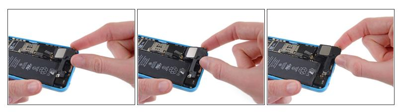
Remove the speaker enclosure. Be careful not to snag it on the antenna cable.
