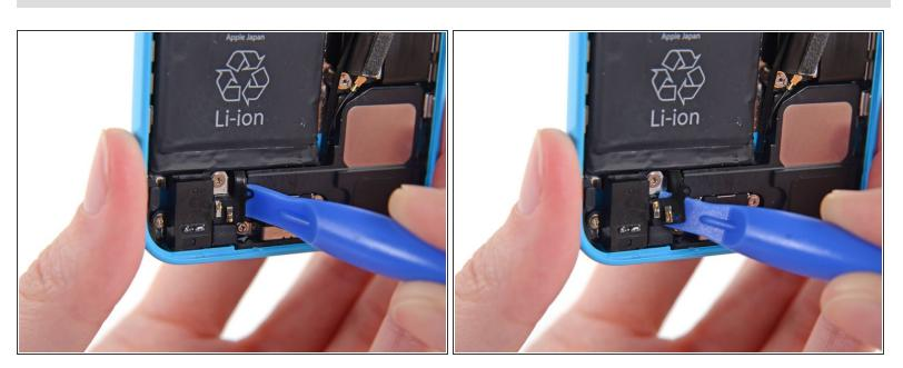
Use a plastic opening tool to peel the home button spring contact cable up from the speaker enclosure.
