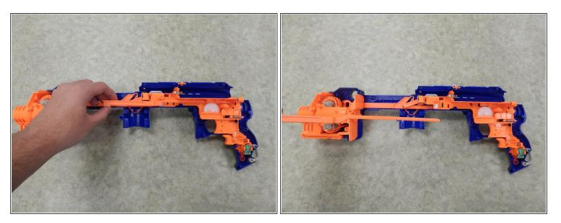
Remove the firing pin.
