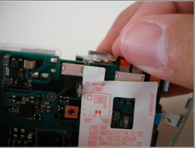
Remove the orange cable connecting the battery terminal to the motherboard.
