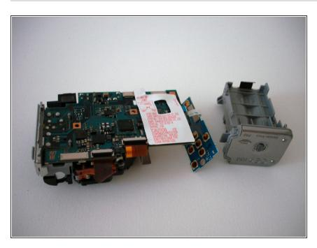
The battery terminal is now free from the board and can be slid out.
