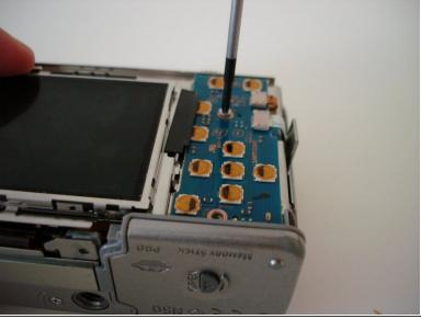
Remove the two screws holding the circuit board down.
