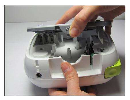
Flip the device over and press down on the indication arrows located at the top center of the back cover and pull it open.
